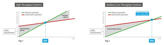
**Fig 1**: The first graph shows that a major investment in an AS/RS system obtains an **attractive return** if the difference between the daily costs of manual operation are significantly higher than the daily costs generated by an **automatic operation**.
